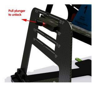
The bottom stop can be indexed on a separate 2pin bar in 8 positions. To change the position of the bottom stop cushion, lift the cushion by using the handgrips and move the cushion forwards or backwards. Choose a comfortable position for the patient and one that stops the patient from sliding down the board.
