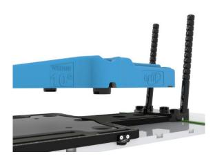
A 15° angle can be obtained by combining the 5° (38103) and 10° (38102) wedge cushions. The 5° wedge cushion should be indexed on the AIO 3.0 base plate and the 10° wedge cushion is indexed on top of the 5° wedge.
