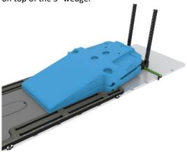
The arm rest low (38106) and high (38100) can be indexed on the 0 degree cushion or the 5° and 10° wedge cushions in exactly the same way by using the indexing knobs already provided in the cushion itself. The indexing knobs will fit into the positioning holes provided in the 0 degree cushion and the base plates or into the positioning holes provided on top of the 5° and 10° wedge cushion.
