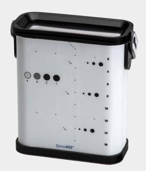
Sono403 Phantoms, with patented HE (High Equivalency) Gel™, provide advanced technology for measuring image quality of small parts and intra-cavity ultrasound scanning systems.
