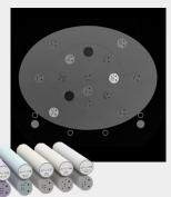
Automatically identifies phantom and location of rods.
