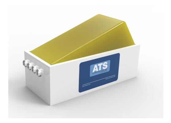
The ATS 523A rubber based tissue mimicking Doppler flow phantoms contain four flow channels of various diameters (normally 2, 4, 6, and 8mm diameter) simulating the deep vasculature of the cardiac and abdominal vessels.
