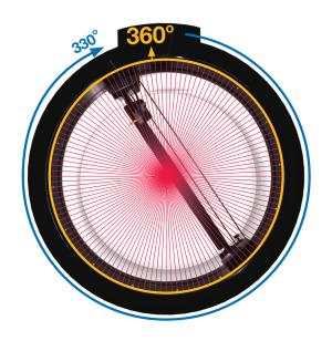
360° of scanning with consistent detector orientation results in better data and eliminates the need to change tank setup.
